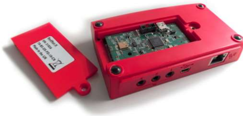
This image shows a RedRat-X with a module fitted inside.
